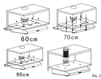
Noice: There are 2 methods for ventilation, including ' horizontal ventilation' and ' vertical ventilation'. Please pay attention to the ventilation method when installation.
