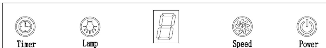
1. Press the “Power” button, the button control the “on” & “off ” of the hood.
