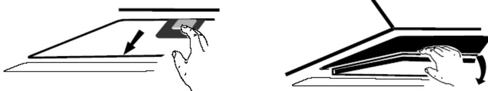
3. Turn the carbon filter on both side of the motor anti-clockwise. Replace the carbon filters with the new carbon filters.
