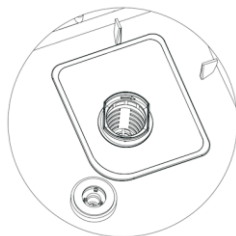
3. Rotate the lifting cup till the lifting cup slot and water tank buckle are fastened.
